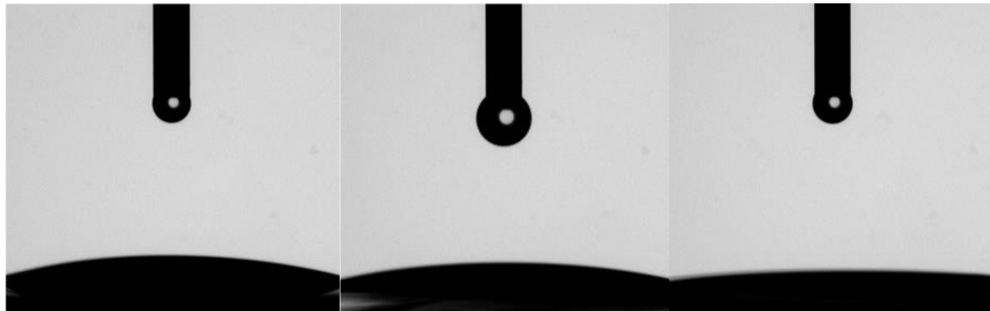
Figure 10. The contact angle of the water/Mo surface. Left – molybdenum cleaning with detergent; middle – surface cleaning with ammonia and alcohol; right – magnetron etching of the surface.
