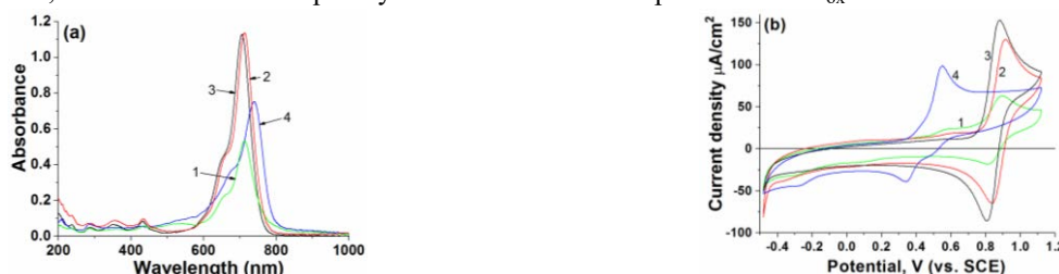
Fig. 2. Absorption spectra (a) and CV curves (b) of indotricarbocyanine dyes in acetonitrile containing 0.1 M TBABF 4 . The curve number corresponds to the dye number in Fig.1.
