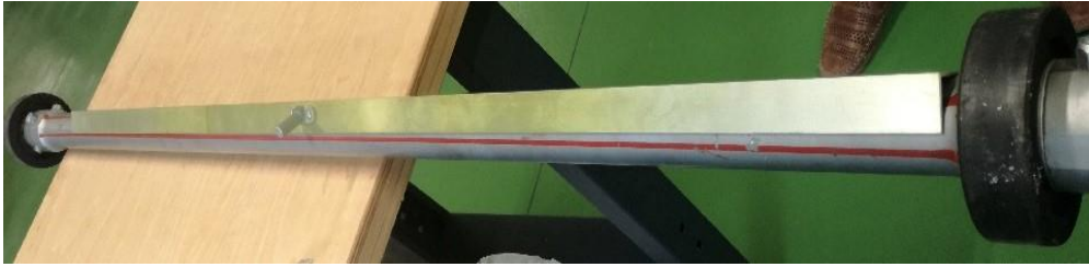
Fig. 4. Twisted rear shaft: 1 - control line applied with paint on the shaft during the manufacturing (renovation) process - visible significant twist of the shaft (approx. 2 mm); 2 - control rule; \beta_1 - angle between the shaft twists
