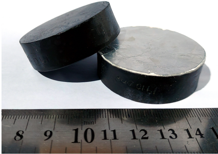
Figure 2.4.2. Bulk single domain seed melt grown YBCO samples. One on the bottom has an aluminum reflector attached.
