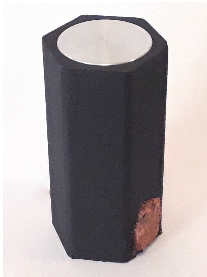
Figure 2.1.3. The launch package used in the experiments of this subsection. The package contains a copper brush armature, a 3D-printed plastic housing and an aluminum disk payload.
