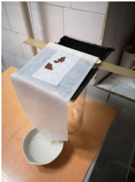
Figure 51. Paraprint OL60 washing of prepared sample
