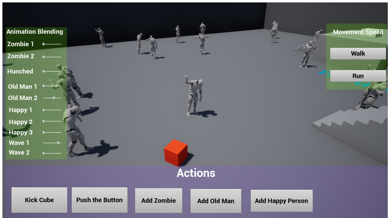
Figure 8. A screenshot of the Unreal Engine 4 animation blending testing tool. Two additive animations (Old Man 2 and Wave 1) are added to the center character animation set at different blend weights, creating new character motions.
