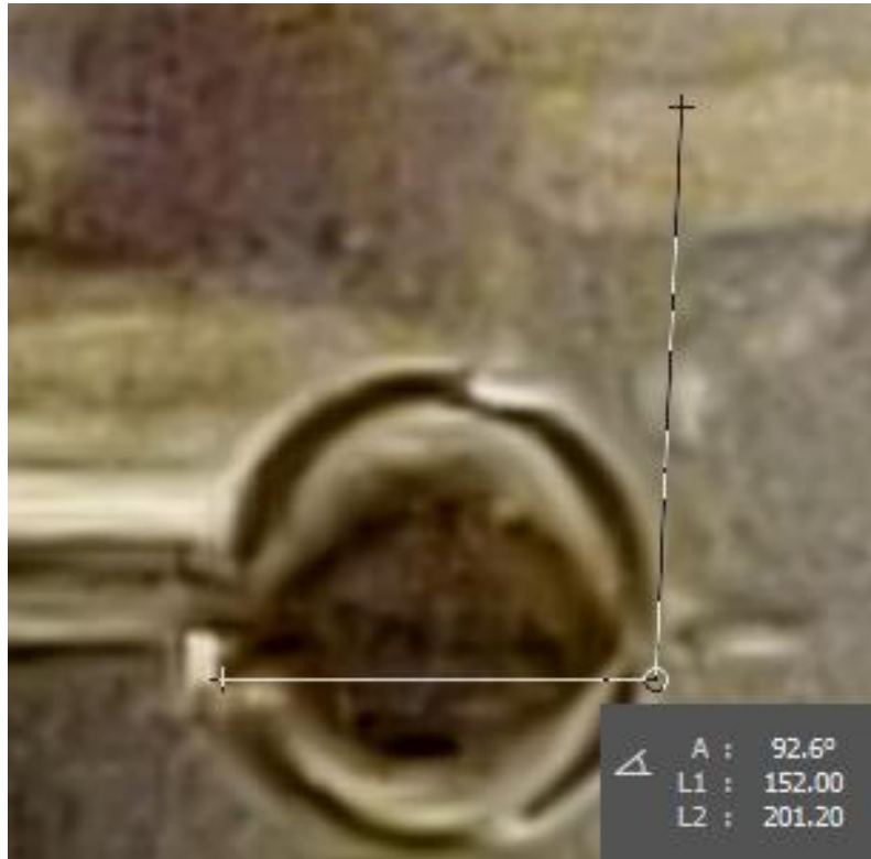
Fig. 25. Water contact angle on glass-ceramic working material on textured and silanized microgrooves. Textured microgrooves are 24\ \mu\text{m} width. 60 iterations. Scanning speed 300 mm/s
