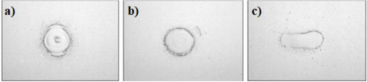
Fig 4. Damaged shape dependence on focus position. a) Focus point is 200 \mu\text{m} above the surface; b) Focus position is on the surface; c) Focus position is 200 \mu\text{m} inside the material. Pulse width: 150fs, wavelength 800 nm, repetition rate 5kHz, pulse energy 0.16mJ [16].
