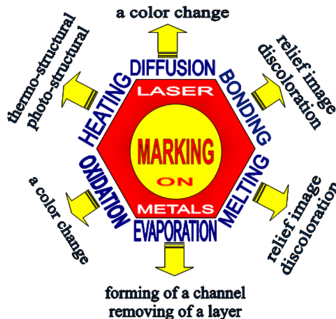
Fig. 1. Physical processes in laser marking. [3]
