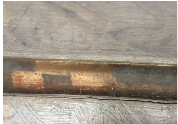
Fig. 1. Uncovering the gilded surface of a painted altar using laser cleaning technology. Exposure of this layer using alternative technologies without damaging the gilded paint layer would be complicated task.
