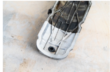
Fig. 2. Engine part with convex and uneven surfaces, covered in grease and soot deposits after laser cleaning procedure.
