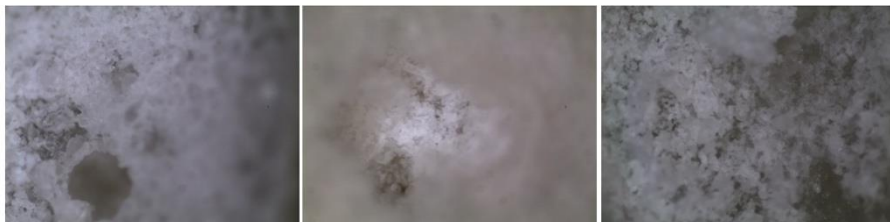
Figure 34. Optical microscopy showing surface morphology and microporous structure of the representative cHAP-PEGDA composite.
