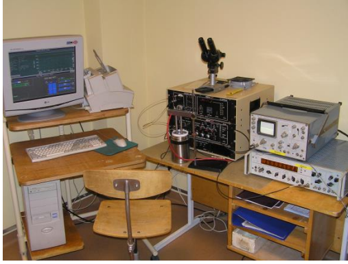
Fig. 3.5. Instrumentation arrangement for DLT spectroscopy using commercial spectrometer DLS-82E.
