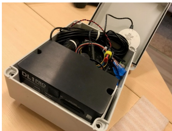
Figure 1: Demonstration of the secured case with DL-1 MK2 Data logger, GPS antenna and additional connector for output connections.
