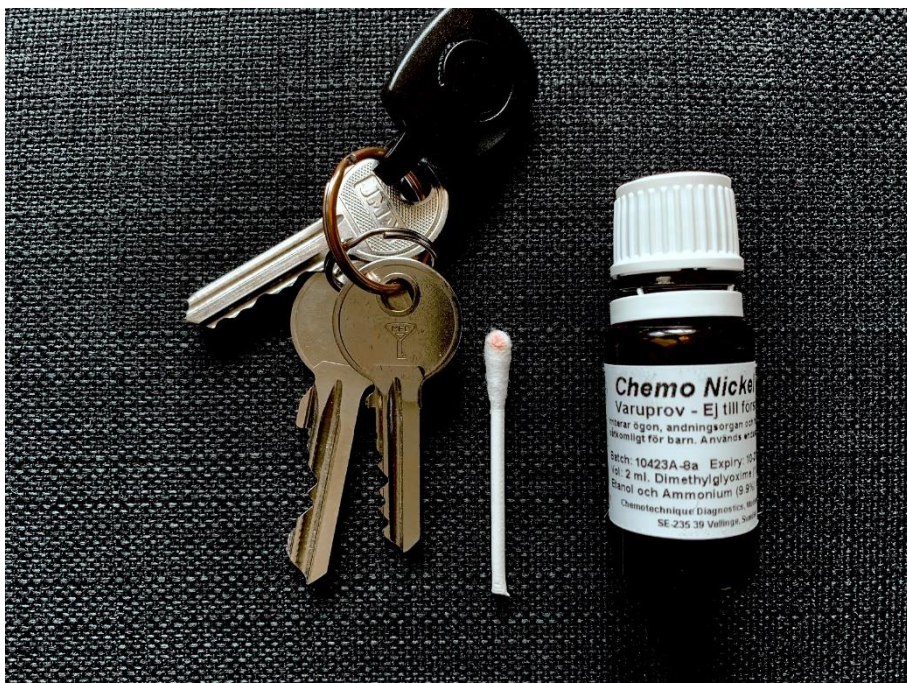
Figure 1. A positive DMG test reaction indicated by the changed color to pink of a cotton stick rubbed the surface of a key.
