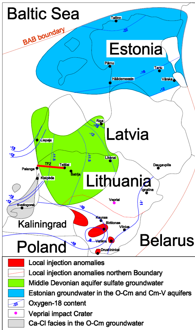
Figure 4.1. Hydrogeological anomalies scheme of the BAB. Local injection anomalies and boundaries – after (Juodkazis et al., 1997). Sulfate groundwater, Ca-Cl facies anomalies, oxygen-18 data in Lithuania and Latvia – after: (Mokrik, 2003), in Estonia after talik scheme (Mokrik & Samalavičius, 2022). TFZ– Telsiai Fault Zone, after (Suveizdis, 1994, 2003).
