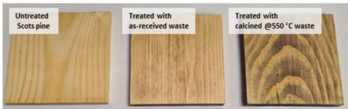
Fig. 9. Camera photos of untreated Scots pine and that of the treated with as-received and annealed at 550°C aquaculture waste material showing different colour of the wood surface due to the deposited material.
