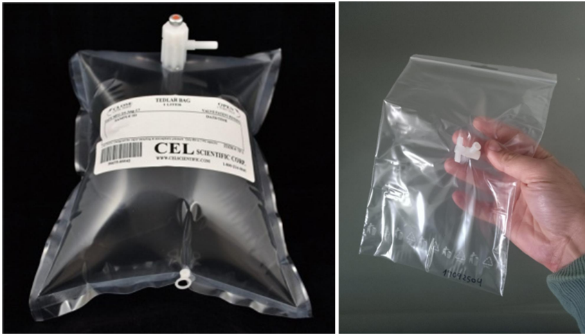
Figure 23: Tedlar ® Bag (Left) and developed Minigrip LDPE plastic bag collection system (Right).
