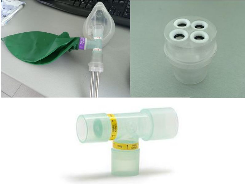
Figure 20: Face mask with 4 sampling tubes (top left); self-made TD tube connector (top right); T-piece directional valve (bottom).
