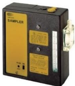
Pav. 2: SKC Inc. Aircheck Sampler 224-44XRM modelis
