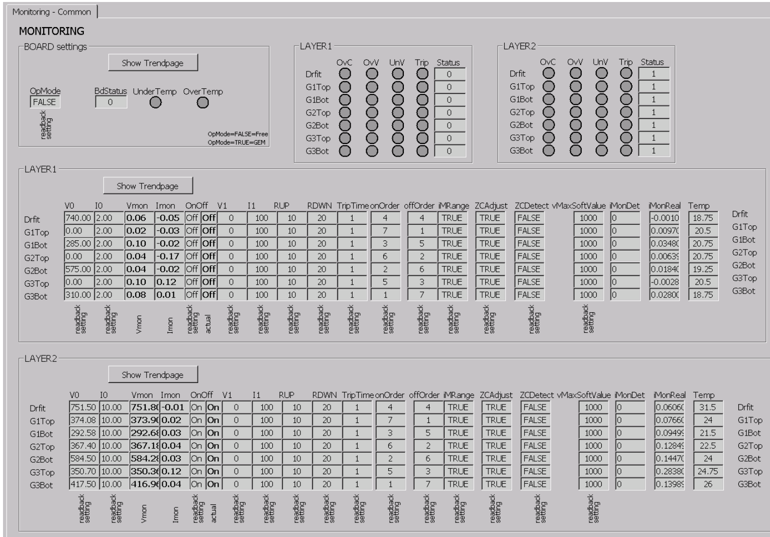
Figure 5. DCS panel for monitoring the actual parameter values of a multichannel power supply.
