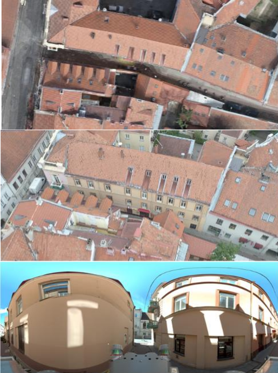
Fig. 9. The first image (Drone mapping – Orthomosaic); The second image (Drone mapping - oblique image); The third image (Mobile mapping – 360 degrees panoramic image)
