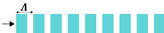
Figure 5. Effective index waveguide. \Lambda depicts period of high refractive index blocks. Arrow shows the mode propagation directions.
