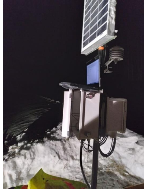
Fig. 3: Installation of mini-RWIS system at Chena Hot Springs Road MP 10 on January 21, 2021. Left: pole-mounting with solar module and weather sensors. Right: mini-RWIS data logger mounted on pole.
