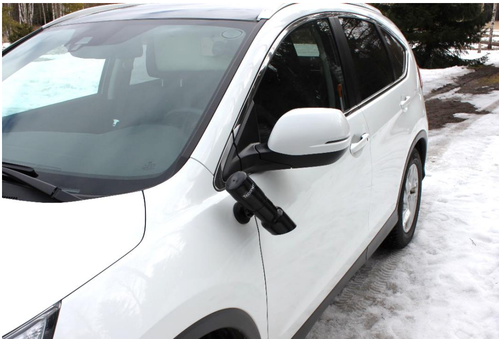
Figure 4. The new compact Road Condition Monitor RCM511 installed by a magnet near the left mirror.
