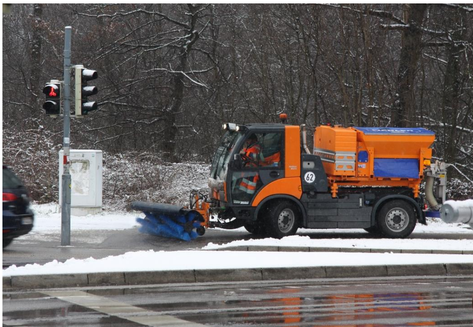
Fig. 3 - Narrow gauge vehicle with front sweeping broom and spreader for pre-wetted salt treatment [picture source Cypra, 2021]
