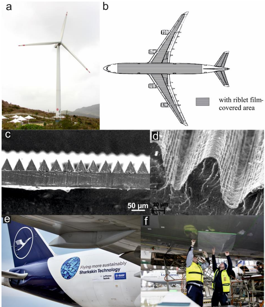
Fig. 18 Industrial applications of shark skin riblets for drag reduction. (a) Wind turbine (author Patrickmak, GNU Free Documentation License); (b) Airbus A340–300 aircraft with riblet film covered area [149]; (c) Riblet film produced by 3M Renewable Energy Division Laboratory tested on aerofoils for wind turbines [146] (reprinted with permission from ASME); (d) Riblets formed by DLIP method on outermost paint layer of aircraft (image rights: 4JET microtech GmbH) [151], (e-f) Lufthansa Cargo’s Boeing 777 should be using riblet film by the year of 2022 (© Copyright Lufthansa Technik) [153].
