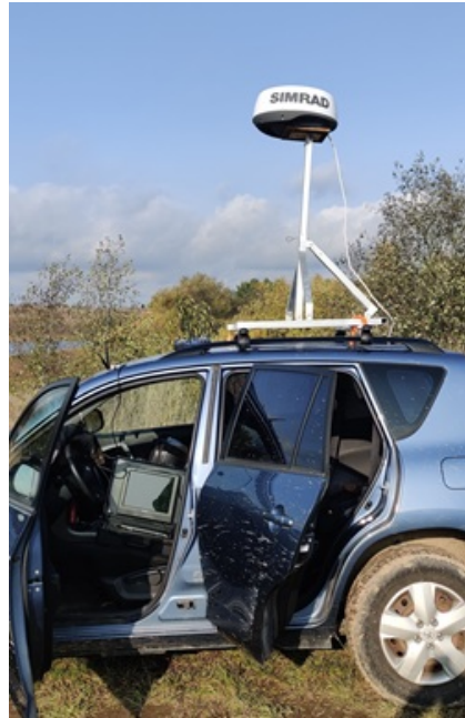
Figure 3. Arrangement of the radar on the car roof.
