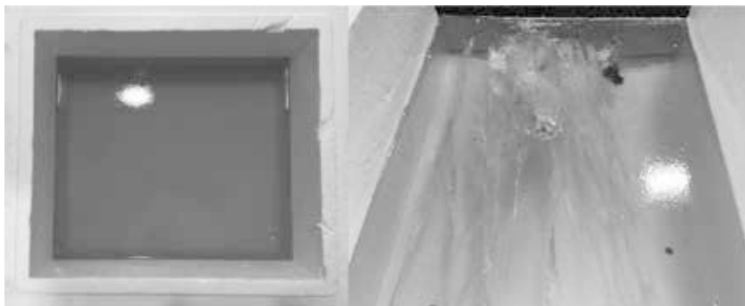
Image 1. A polystyrene container with pure ballistic gelatin (A) and after the shots have been fired (B). Source: authors.
