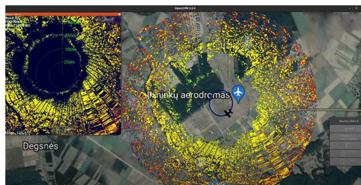
Figure 10. Clutter estimation during a flight on a circular trajectory.
