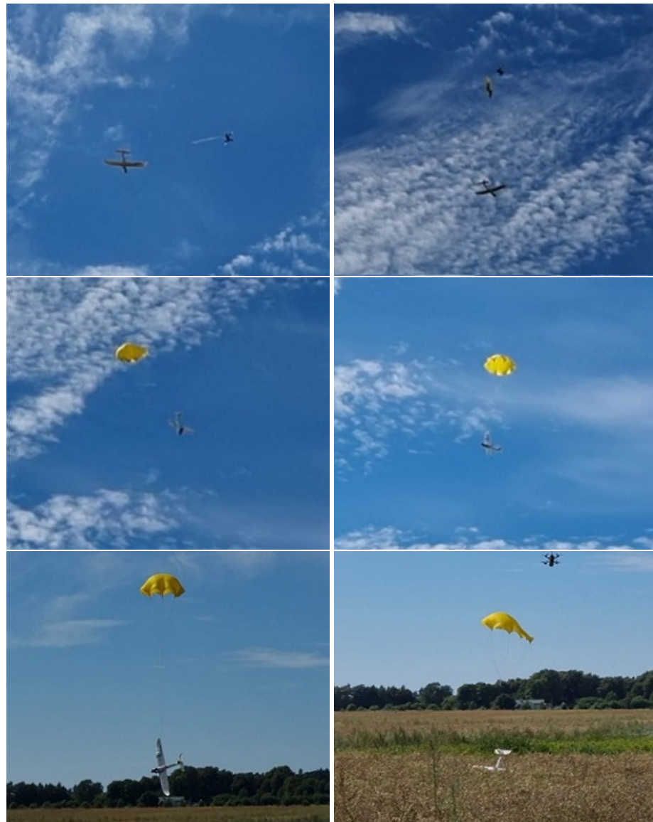
Figure 16. Neutralizing of the fixed-wing UAV.
