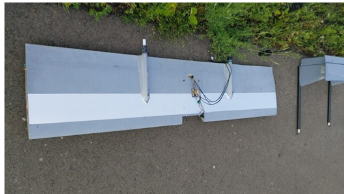
Figure 6. Band of reflective vinyl film on the underside of the wing.
