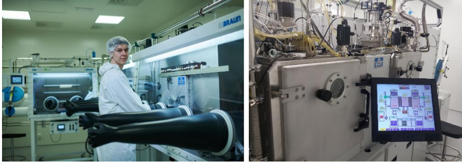
Fig. 4 The author of this dissertation in cleanroom facility and vacuum evaporation system back-end side.
