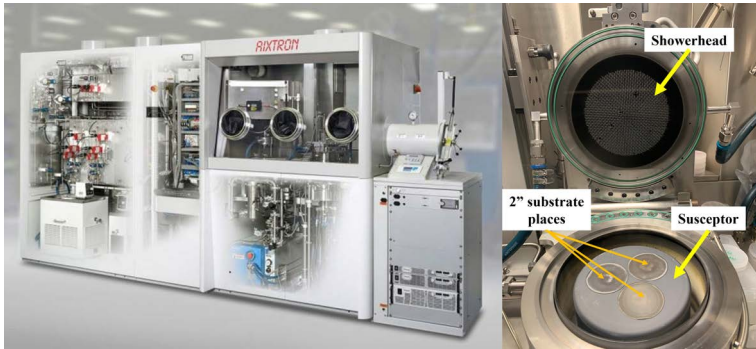
Figure 3.1: Aixtron Ltd. 3x2" CCS reactor and reactor chamber. Left-hand picture adapted from [66].
