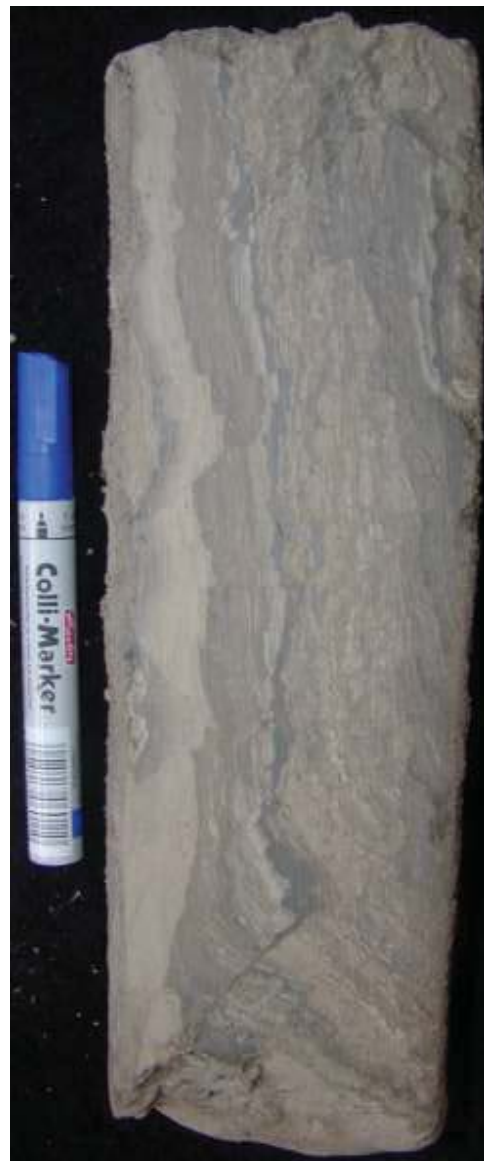
Fig. 2. Core of borehole from Klaipėda Strait: glaciодislocated inter-till micro-layers of clay, silt and silty sand (photo: A. Damušytė).
