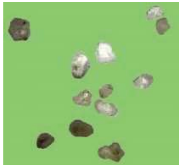
Fig. 4. A solid color background created in the Color Analysis window of the Surface Photo Model program.
