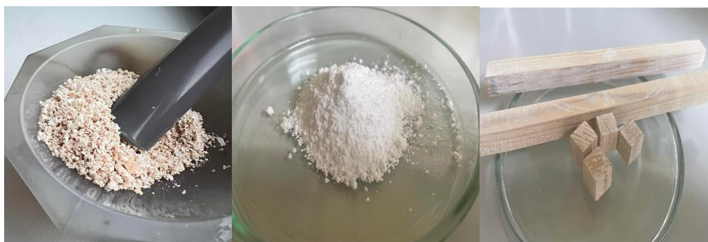
Fig. 1. Photos of grinded waste eggshell (left), \text{Ca}(\text{OAc})_2 produces from eggshells (middle) and successfully mineralized pine wood with calcium phosphate bioceramics (right).
