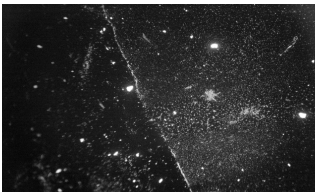
Fig. 2 . Length of this picture is 0.8 mm. Diameter of precipitations of carbon on silicon in the irradiated right side is about 1 \mu\text{m} . Left side is not irradiated.
