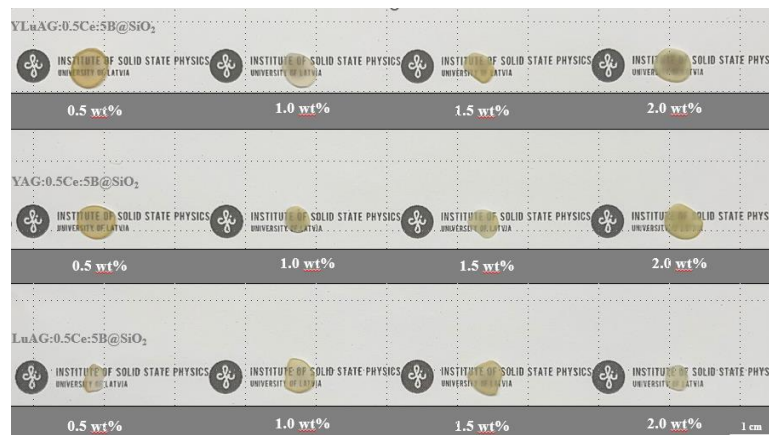
Fig. 1. Photo of samples with different concentrations of phosphor: YLuAG:0.5 % Ce@SiO 2 , YAG:0.5 % Ce@SiO 2 and LuAG:0.5 % Ce@SiO 2
