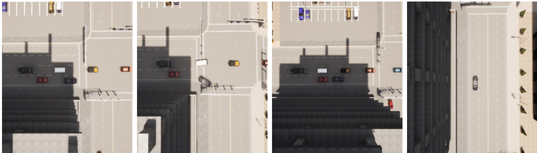
Figure 8: Example images where ego vehicle (gray) correctly passes intersection (1st and 2nd image from the left) and where it fails to start driving (3rd and 4th image). Examples are taken from test runs with PMW-query model.
