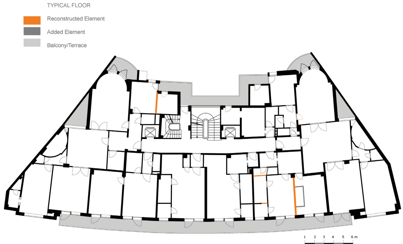
Fig. 6: "Central Palace", typical floor plan. Source: Rocom, PMB, drawing after the surveying plans.
