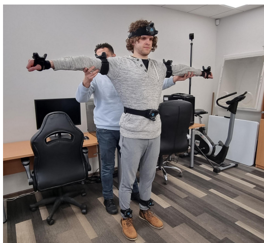
Figure 6. Assignment of sensors to body parts during calibration of the BiomacVR system. A person is assisted by a nurse.
