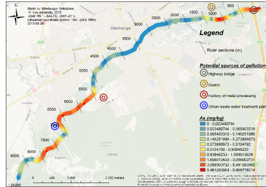
Fig. 5. The distribution of arsenic (As) concentrations in the river of Sventoji bottom sediments at the city of Ukmerge.
