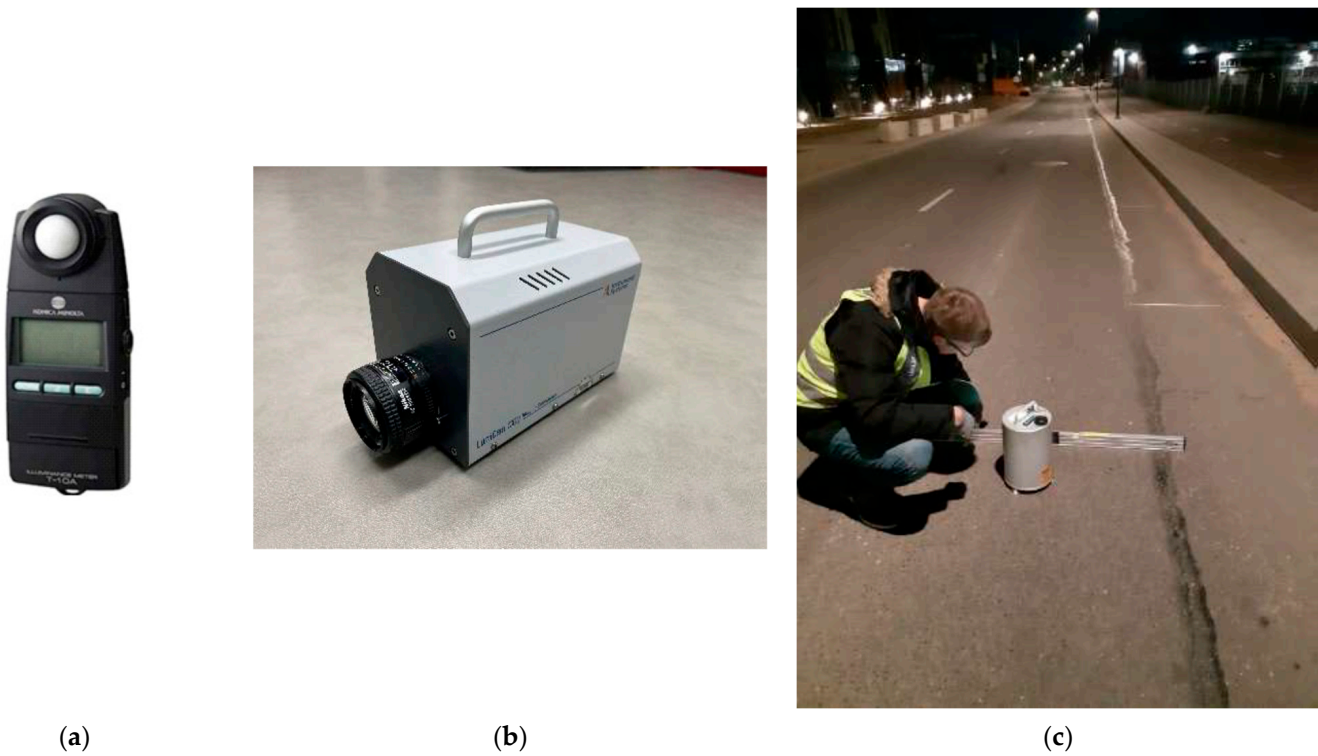
Figure 4. Devices used for the experimental study: (a) lux meter, (b) LumiCam 1300 camera, (c) digital spirit level and laser profilometer.
