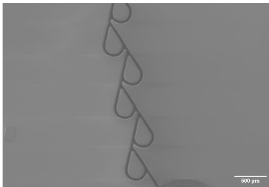
Figure 7. SEM image of final Tesla valve before sealing.
