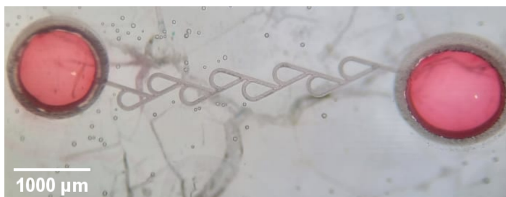
Figure 8. Optical microscope image of Tesla valve testing for any leaks by injecting red-colored water. No leaks or blockages can be detected, showing superb sealing through the whole cm-sized chip.
