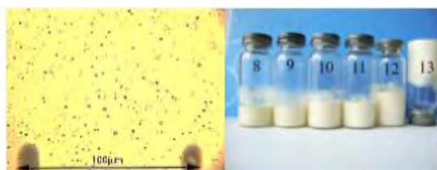
Fig. 3. a – Micrograph of lavender oil solubilized with a pseudopolyamino acid dispersion, b – photo of samples of the polymer-stabilized m/w emulsion.
