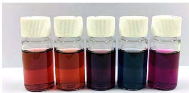
Fig. 1. AuNRs of varying lengths were produced using the seed-mediated method.
