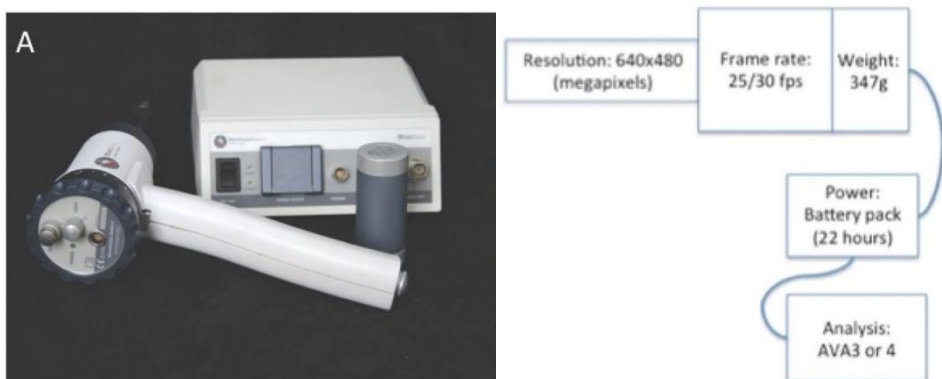
Figure 4. Photograph of side stream dark field camera and characteristics Adapted from Coppel et al. [90]
