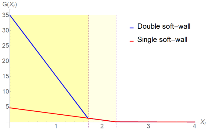
Figure 6.2: Single (6.19) and double “increase–increase” (6.20) force G profiles for k_1 = 0.001, k_2 = 2, k_3 = 20, a_1 = 2.3, a_2 = 1.7 .
