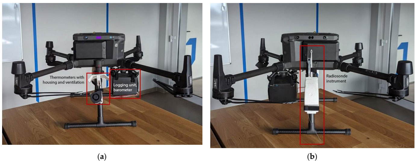
Figure 2. Illustrates the mounting of instruments onto the DJI M300 drone. Subfigure (a) presents the TMP117 and SHT41 sensors' housing and ventilation unit as illustrated in Figure 1, as well as the logging and barometer unit. Subfigure (b) shows mounting of the RS41 sensors.
