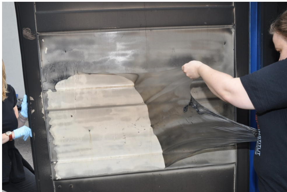
Figure 4. The pulling of a latex membrane in an experimental setup. This method can be applied to samples of all sizes.
