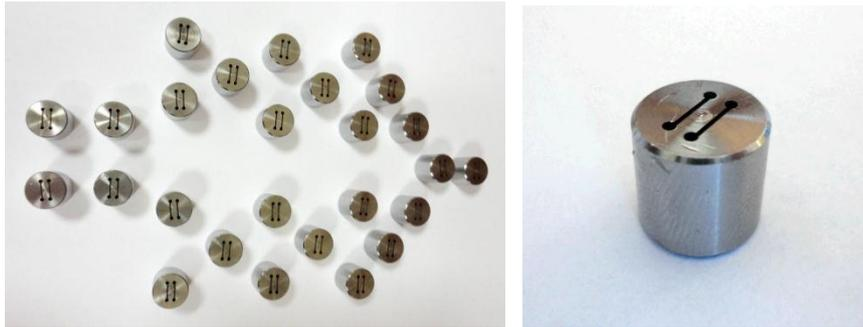
**Fig. 3.9** Samples prepared for ceramic mesh fabrication. Two separate, parallel grooves were fabricated on the surface of the steel sample, with dimensions  $350 \times 300 \mu\text{m}$  and  $310 \times 500 \mu\text{m}^2$ .
