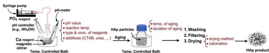
Fig. 10. Preparation of CHAp nanoparticles via chemical precipitation.
