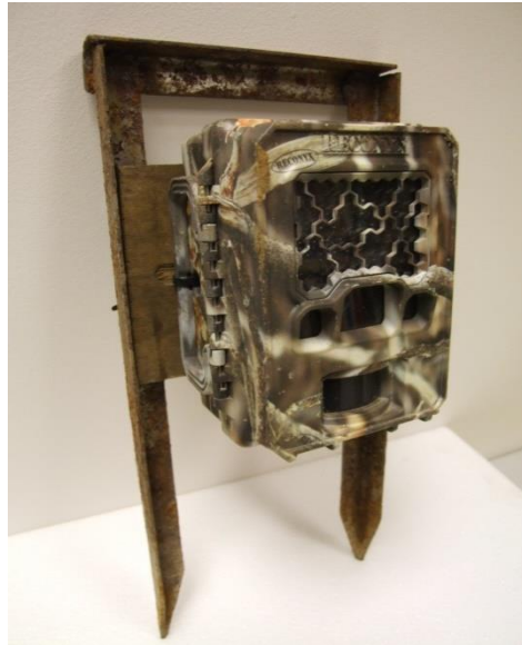
Figure 14. Camera fixed on the platform ready to be installed into a beaver burrow (photo by A. Ulevičius).
