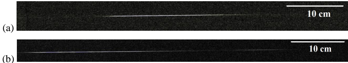
Fig. 1.3.1. Experimentally registered filaments. Energy 1.5 mJ (a) and 2.2mJ (b), pulse duration 35 fs, f = 2000 mm. (b) picture illustrates the refocusing of the FH beam.
