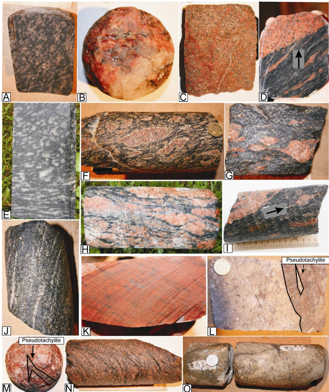
Fig. 2. Macroscopic classification of the investigated rocks within the TDZ: Weakly deformed rocks: A) Charnockitoid (Mikoliškės-1); B) Pegmatite (Genčiai-6); C) Fine grained granite (Genčiai-6); Mylonites: D) The contact of charnockitic mylonite with weakly deformed fine grained granite (Genčiai-6). Black arrow shows a top of drill core; E) The contact of weakly deformed and mylonitised charnockitoid (Mikoliškės-1); F) Augen mylonite of charnockitoid (Kretinga-4); G) Augen mylonite of charnockitoid composition with boudinaged veins of granite composition (Kretinga-1); H) Coarse grained granitic mylonite (Genčiai-6); I) The contact of a mylonitised charnockitoid with coarse-grained granite (Genčiai-6). Black arrow shows a top of drill core; J) Mylonite of charnockitoid with ribbon structure (Nausodis-3); K) Metapelitic ultramylonite (Girkaliai-2); Cataclasites and pseudotachylite: L) Breccia with pseudotachylite in charnockitoid (Kretinga-3); M) Pegmatite with pseudotachylite (Girkaliai-2); N) Cataclased charnockitoid (Genčiai-11); O) The brecciated contact of the charnockitoid with the Cambrian sandstone (Genčiai-3). The diameter of drill cores is 7.8 cm.
