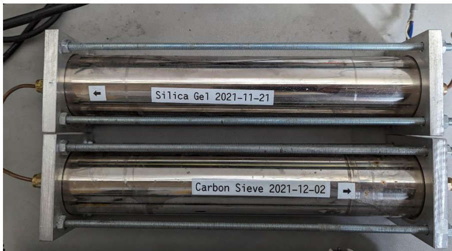
Figure 35. Photo of the custom H 2 carrier gas drying filter.
