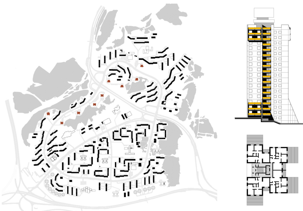
Fig. 4. Lazdynai , 1969–1981, arch. V. E. Čekanauskas, V. Brėdikis and Č. Mazūras. On the left – the site plan with concrete towers marked in brown; on the right – the façade and plan of a concrete tower [drawings by Aušra Černauskienė].
