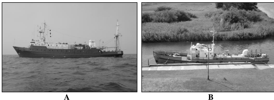
Fig. 2.2.1.1. Research vessels of the Center of Marine Research: A – research vessel “Vėjas” for the national monitoring of the Baltic Sea (1980–2009; length: 55.6 m; width: 9.3 m; draught: 4.3 m; 7 laboratories; 12 crew members; 20 members of scientific group); B – expedition boat of for the national monitoring of the Curonian Lagoon (1983; length: 21 m; width: 4 m; draught: 1.6 m; 1 laboratory; 2 crew members; 5 members of scientific group)
