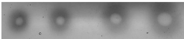
Fig. 3 Functional analysis of Novozymes® 51,003 laccase on the agar plates containing 4.5 \mu\text{g ml}^{-1} Ferbamine. Amount of the enzyme added, from left to right: 1, 2, 3, 4 \mu\text{l} . Incubation conditions: 20 h at 20^\circ\text{C}
